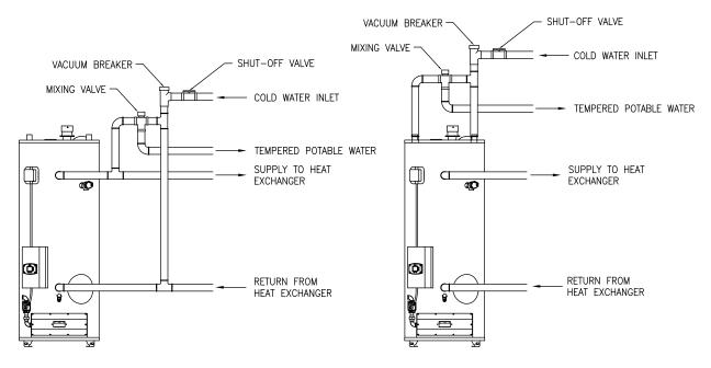
Suggested Piping Arrangement For Side Connections
